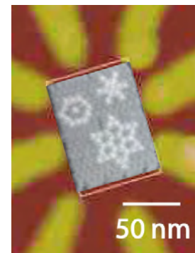
Figure 3. An AFM image of a DNA-origami structure superimposed, to scale, on an SEM image of eight gold nanowires.
