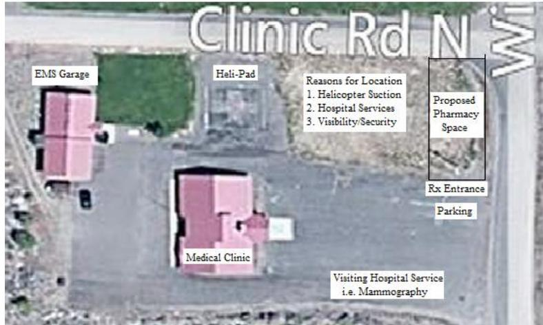
The location of the pharmacy was determined for several reasons. The helipad prevented the pharmacy from being located closer to the building out of fears of roof damage from the suction created by the helicopters rotors. The south side of the property is currently set-up to accommodate visiting medical services such as mobile mammography. The best location was determined to be in the site shown. This site is part
