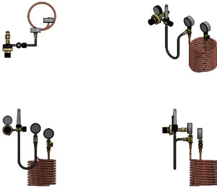
Figure 4: Parts and assembly drawings of the argon condenser prototype
