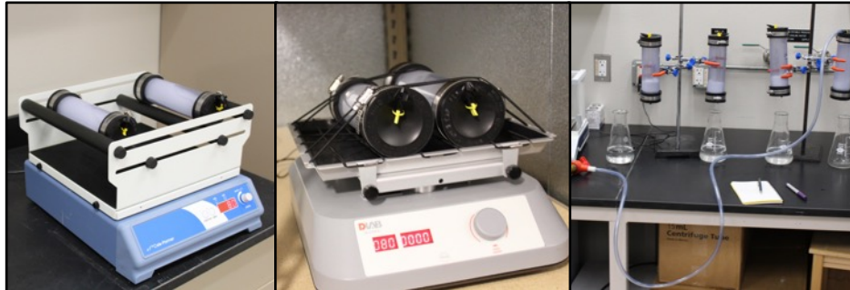
Figure 2. Images of the weathering chambers on the shaker tables and in the drain stand setup.
