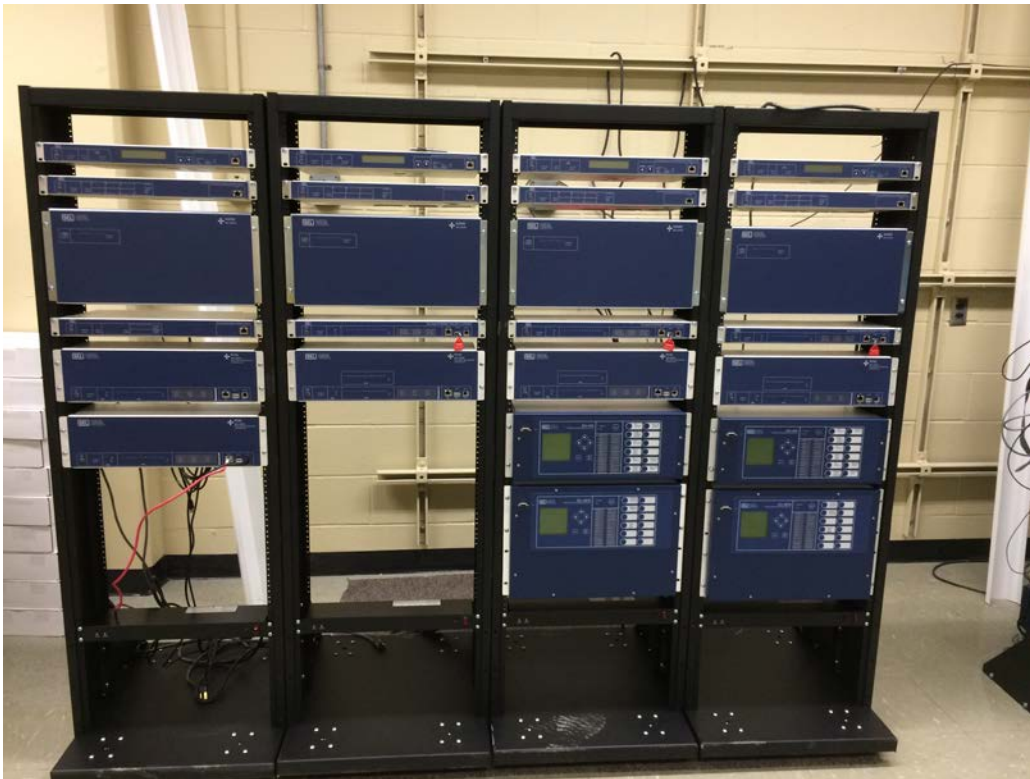
Figure 6: Some of the test equipment for the expanded PowerLab along with new equipment racks (each rack will simulate a complete power substation's control).
