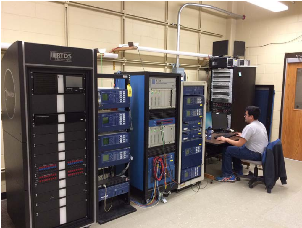
Figure 7: PowerLab Component of the ICS Testbed with the addition of the new RTDS NovaCor rack (to the left).
