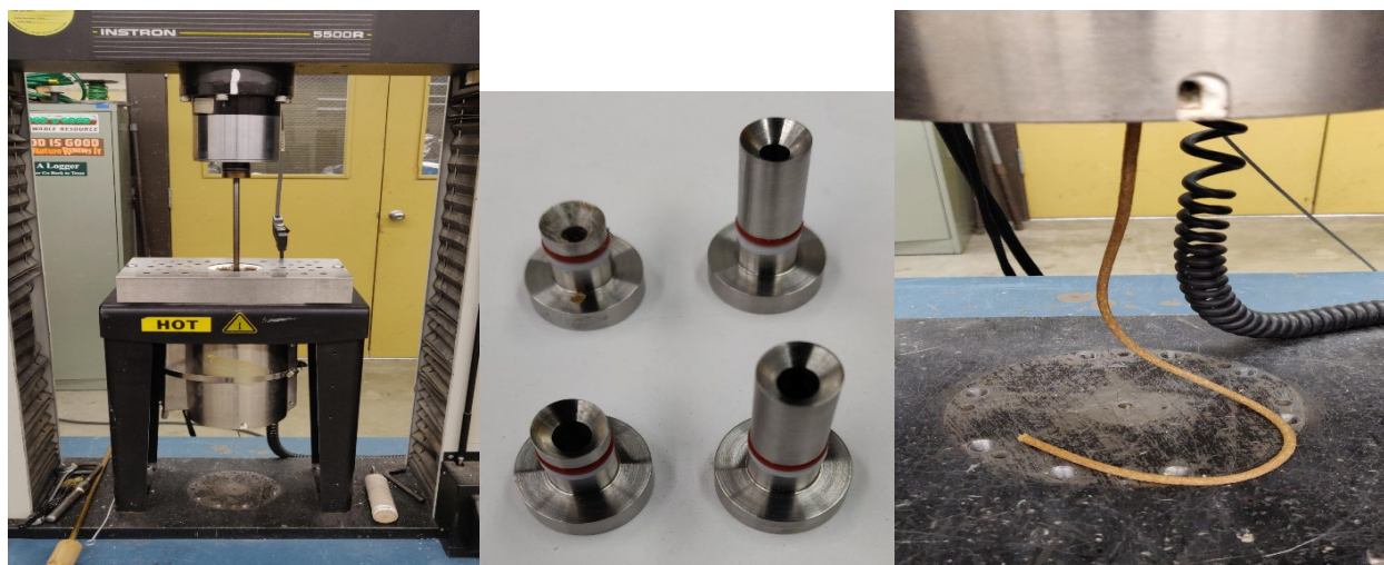
Figure 3. (left) Capillary rheometer, (middle) dies used, and (right) extruded wood/resin mix through die
