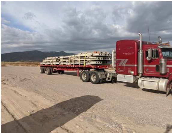
(c) Transfer of precast concrete sections
