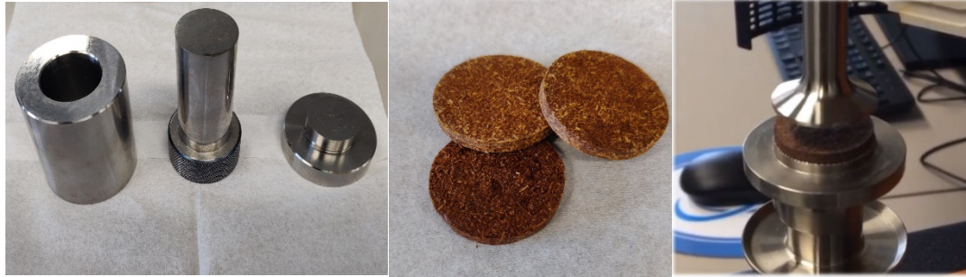
Figure 1. (left) pellet press die (25 mm), (middle) pressed samples, (right) sample loaded onto rheometer
