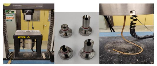
Figure 3. (left) Capillary rheometer, (middle) dies used, and (right) extruded wood/resin mix through die
