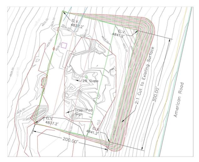
Figure 4. Cut and Fill plan of the outdoor training facility
