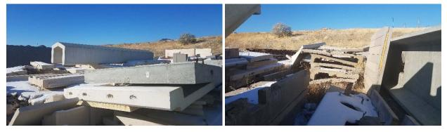
Figure 6. Precast concrete waste pile at Forterra Structural Precast Concrete in Salt Lake City
