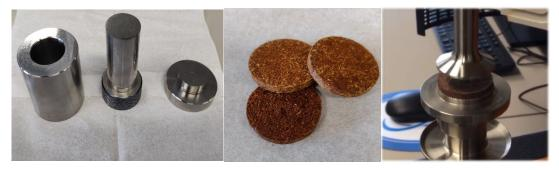
Figure 1. (left) pellet press die (25 mm), (middle) pressed samples, (right) sample loaded onto rheometer
