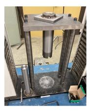
rheometer and a load frame. The scale this technique up, UI ME has designed and fabricated a larger format rheometer barrel and frame. To implement this technique, the wood mixture is loaded into the barrel, then the plunger is inserted into the barrel. The load frame then applies load to the plunger, compressing and extruding the wood mixture out the nozzle at the bottom of the barrel. The direct extrusion frame positioned on the base of the load frame (outside of image) is shown in Fig. 2.
