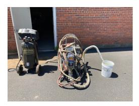
Figure 3. Commercial exterior texture sprayer
