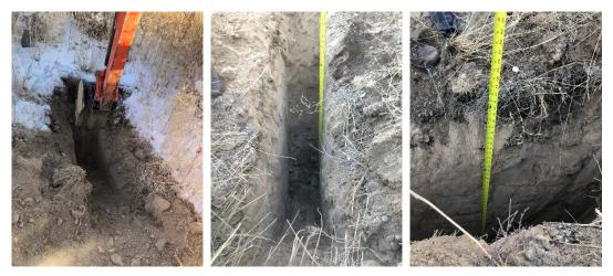
Figure 3. Test pits for soil sampling
