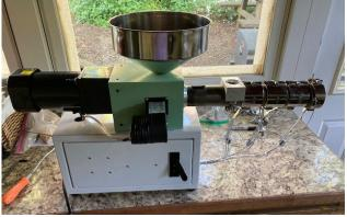
Figure 1. SJ-35 screw extruder with modifications.
