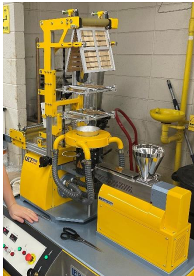
ii. Figure 1. Photo of blown-film being produced of polylactic acid-PHBV blend
