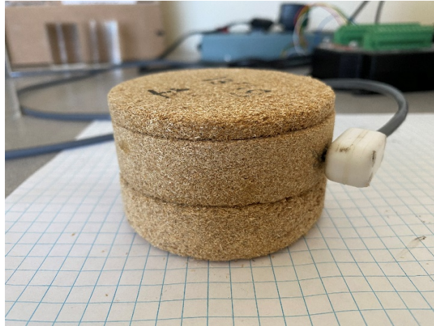
Figure 6. Thermal Testing Using a Transient Probe Method.
