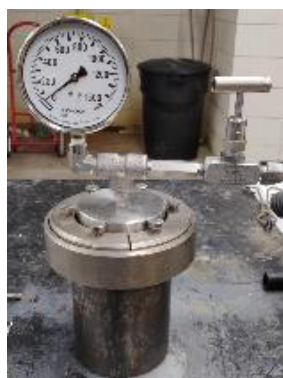
Figure 3: Pressure vessel used for \text{CO}_2 curing
