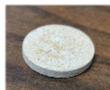
c) After \text{CO}_2 (60 psi and 60^\circ\text{C} ) and thermal curing
