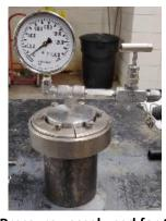
Figure 3: Pressure vessel used for CO<sub>2</sub> curing
