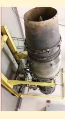
program and is used to test the Matlab™ program. Center. This is the compressor that is modeled in the SolidWorks™ University's Measurement and Control Engineering Research This is the Westinghouse J34 jet engine housed at Idaho State
