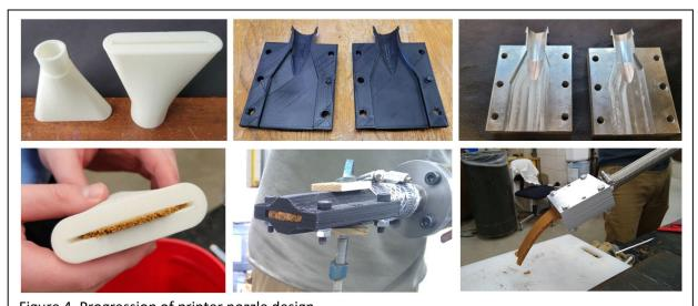
Figure 4. Progression of printer nozzle design.
