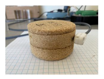
Figure 6. Thermal Testing Using a Transient Probe Method.
