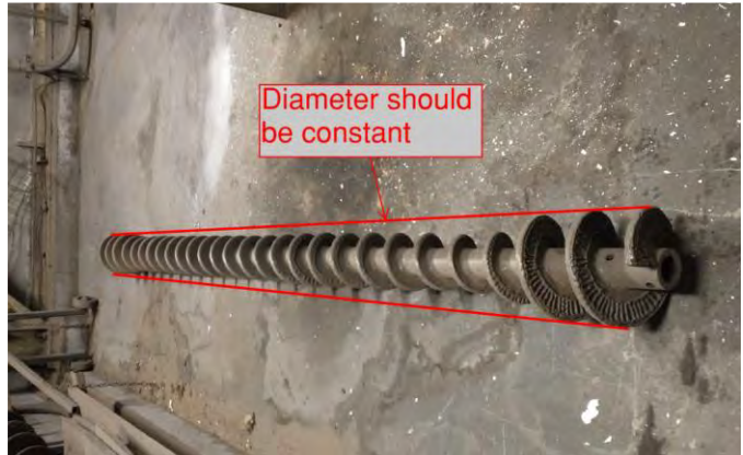
Figure 3. Heavily worn ash augers, significantly reducing performance.
