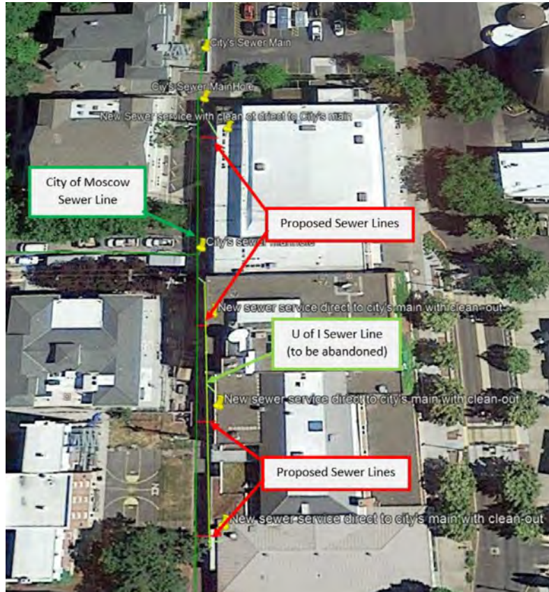
Figure 1. Sanitary sewer system in affected area.
