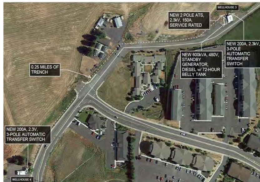
Figure 1. Electrical site plan.
