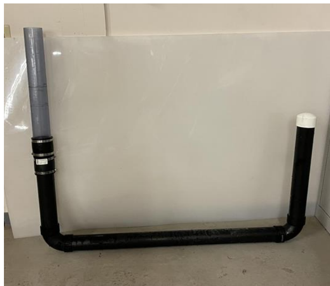
Figure 18 Falling Head Permeability Test Apparatus
