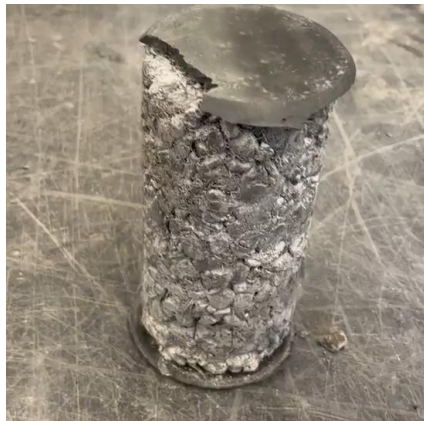
Figure 22 Traditional Pervious Concrete with Fibers Fracture
