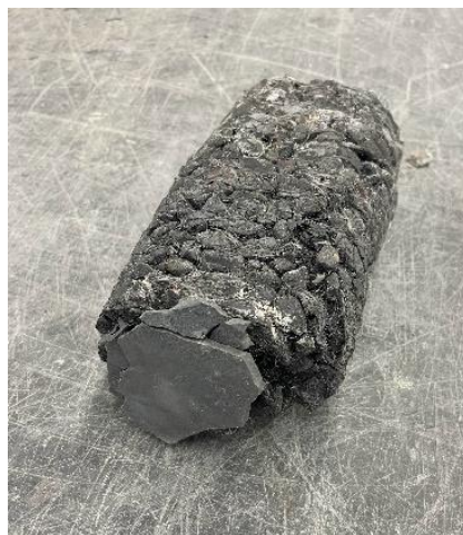
Figure 23 Traditional Pervious Concrete with Fibers Loaded Laterally
