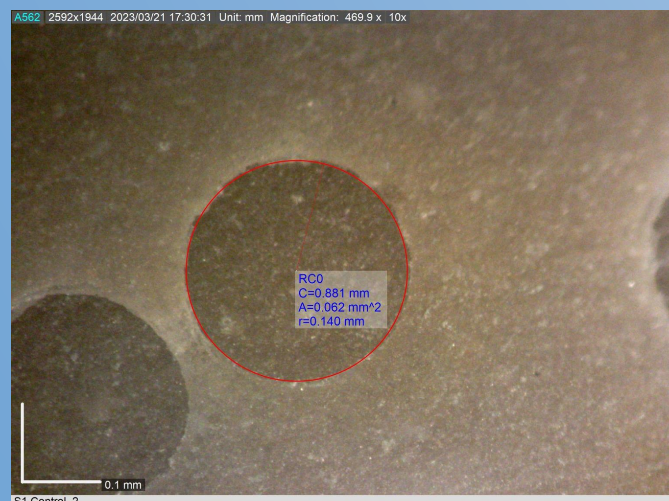
Figure 2. Leeb Round Hardness Test indentations on chert matrix.
