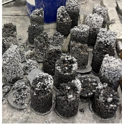
Figure 21 Traditional Pervious Concrete Fracture
