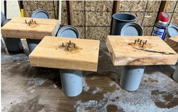
Figure 17 Method to Form Pervious UHPC
