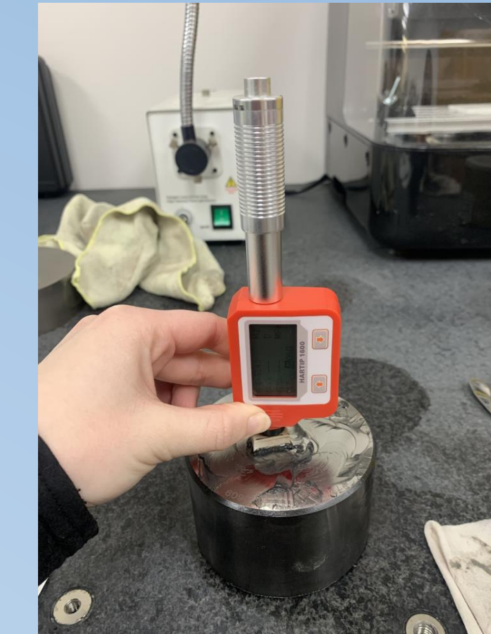
Figure 7. The LRHT apparatus being used on one of the samples.
