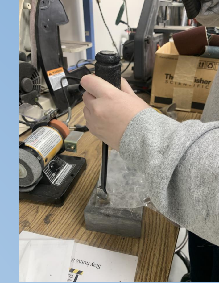
Figure 8. This is the method in which the chert samples were cleaved for the profilometry.
