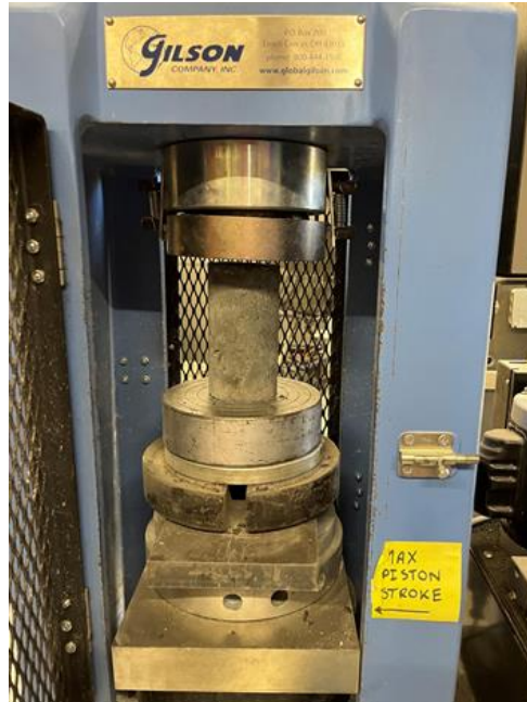
Figure 19 Compressive Strength Test Apparatus
