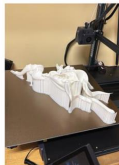
Attachment on the 3D printer in PLA filament. Buildplate dimensions are 420 x 420 x 500 mm
