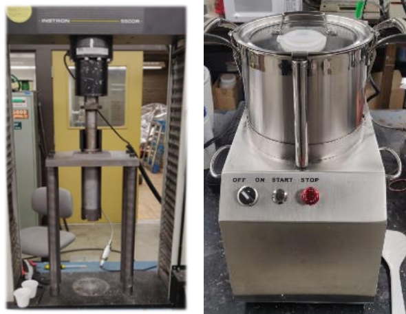
Figure 2: a) Large Capillary rheology setup and, b) Industrial food processor.
