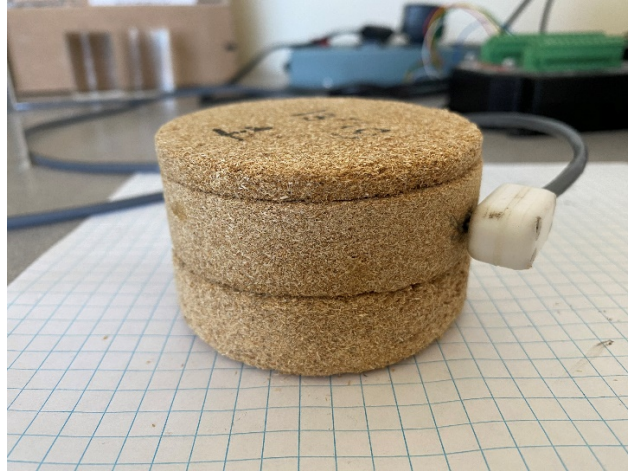
Figure 6. Thermal Testing Using a Transient Probe Method.
