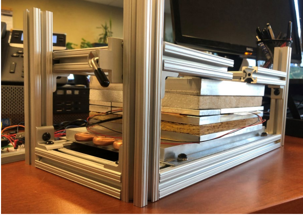
Figure 2. Guarded Hot Plate used to examine the thermal properties and to set up a testing protocol for future samples based on ASTM standard C518
