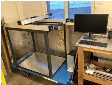
Figure 3. 3D printer frame and gantry system
