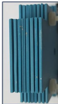
Figure 5. Pictorial drawings and images of our (left) planar CAP array and (right) radial CAP array for killing and removing pathogens from surfaces in food processing.
