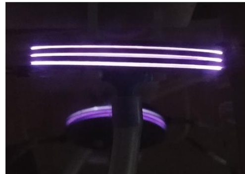
Figure 5. Pictorial drawings and images of our (left) planar CAP array and (right) radial CAP array for killing and removing pathogens from surfaces in food processing.
