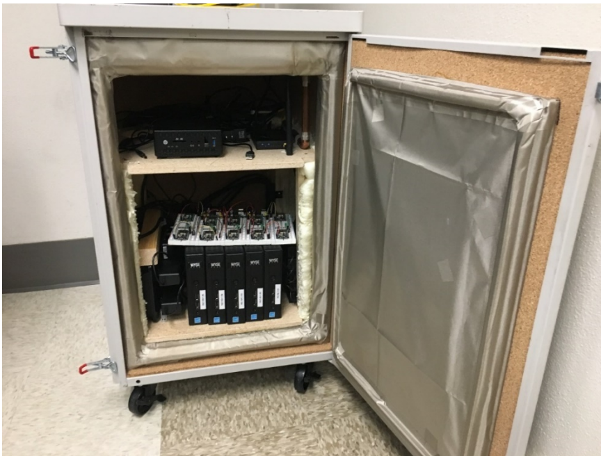
Figure 10: The RADICL-Moscow Cybersecurity laboratory Small Faraday Cage.
