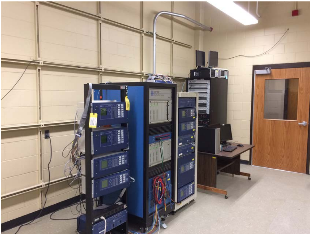
Figure 5: RTDS, some of the test equipment racks and power amplifiers in the remodeled PowerLab space
