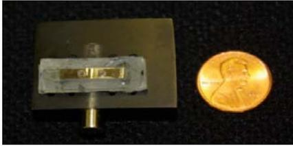
**Fig. 3 MSM pump in jig with diametrically magnetized cylindrical magnet.**
