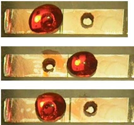
**Fig. 4 MSM micropump moving colored aqueous solution**
