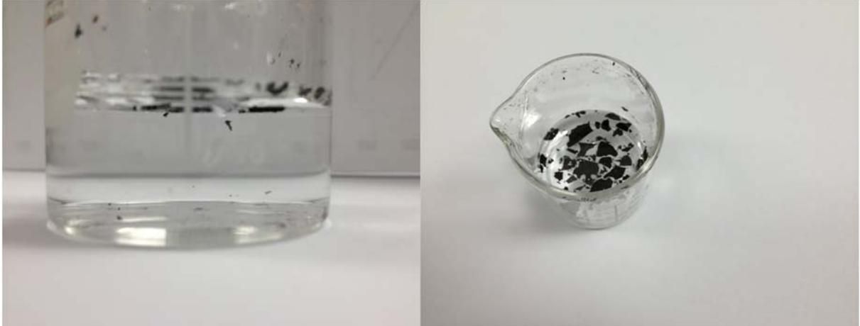
Figure 2. Graphene from silicon wafer A in water, before oxidizing.
