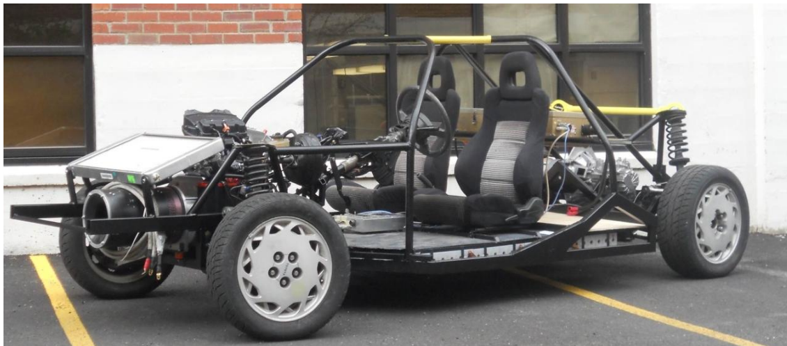
Figure 8 University of Idaho Plug-in Hybrid Electric Vehicle with Horizontal Plate Batteries
