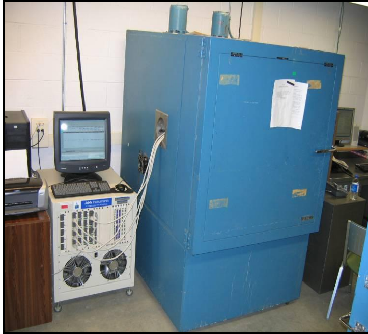
Figure 7 Low Power Arbin Test Station
