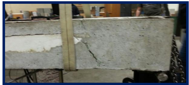
b: Shear Failure – Diagonal Crack
