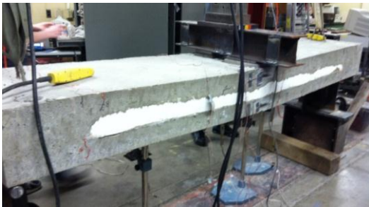
k: Panel Failure
