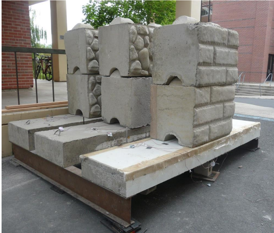
Figure 7: Creep Test Set-up
