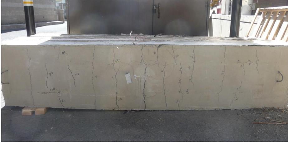
Figure 24: Bending Failure Crack Pattern
