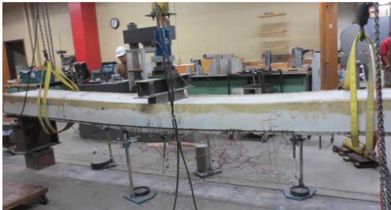
Figure 28: Bending Failure
