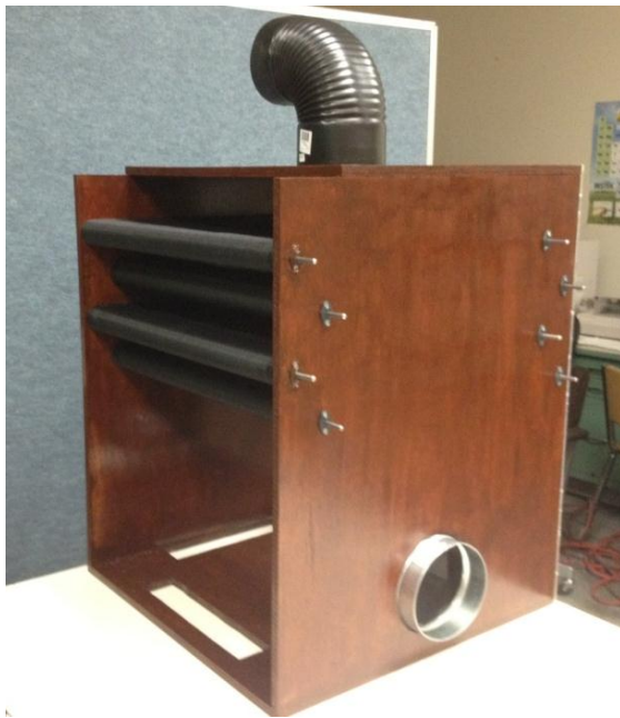
Figure 4: Prototype of conveyer belt type BioEx bead dryer.
