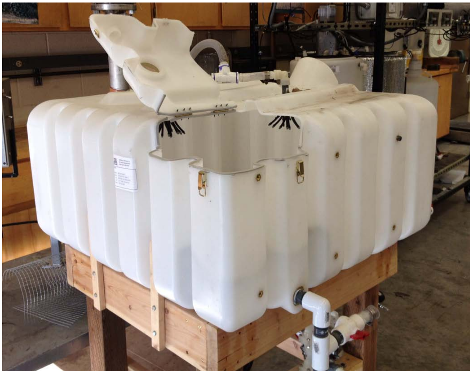
Figure 1: Pilot scale sprinkling type fermenter
