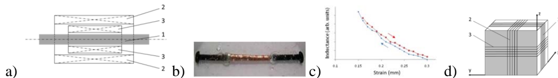
Figure 2: MSMA-based sensor; a) schematic of the 1D sensor; (b) proof-of-concept 1D sensor; the length of the coil is about 1 cm; (c) preliminary results showing a strong effect of the deformation of the MSM element on the inductance of the coil; (d) schematic of the 3D sensor.
