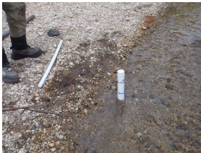
Figure 7. Field temperature probe installation, South Fork Boise River.
