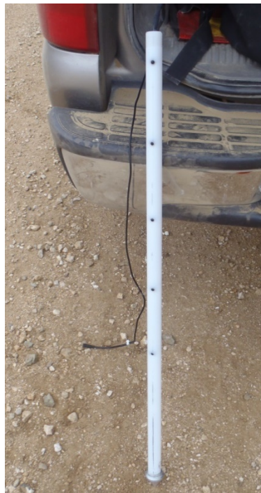
Figure 6. Field temperature probe.
