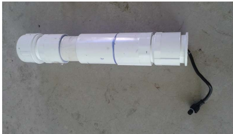
Figure 7. Field temperature probe data logger.
