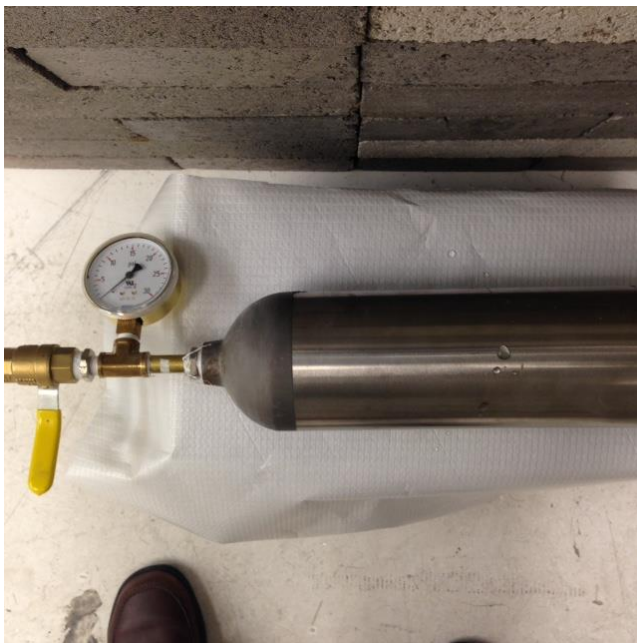
Figure 4 Evacuation tank. The Xe gas is very expensive and after production most of the Xe remains for future use. The tank holds the Xe after use.
