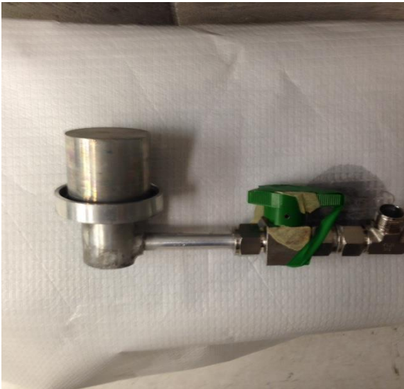
Figure 3 Target after use in the system. The large aluminum cylinder held the Xe for activation by the accelerator. The green valve is for transferring the gas.
