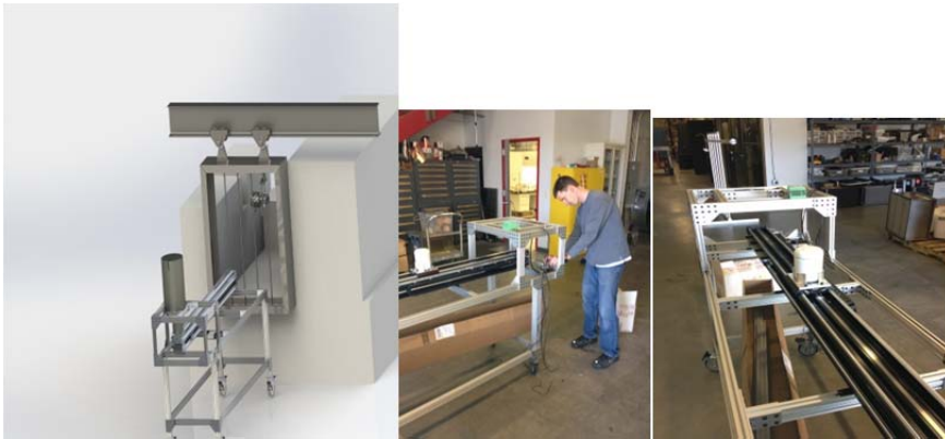
Figure 7 - Left picture is the designed handling system to remotely remove the production product, the center and right pictures are of the constructed handling equipment.
