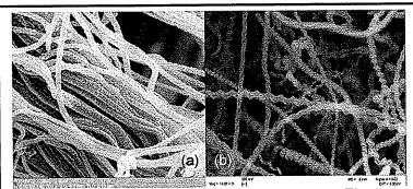
**Figure 3.** Field Emission Scanning Electron Microscope image of (a) knee joint collagen and (b) silica nanosprings. Both images at 14000 X.
