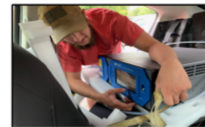
Figure 2. Eli Moser calibrating the T102 sulfur analyzer.
