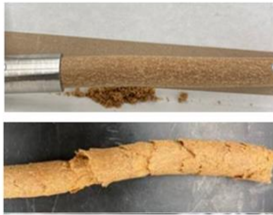
Figure 2. Photographs of (a) smooth extruded wood-SS (50:50) rods and (b) extruded wood-SS showing sharkskin.
