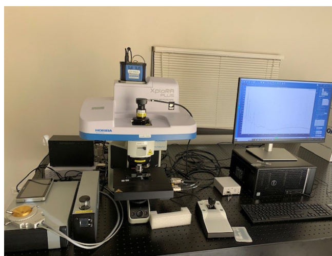
Fig. 54 Confocal Raman Microscope (Horiba, XPloRA Plus) with a Linkam Hot stage. Raman spectra can be obtained in-situ while heating the samples to 1100\text{ }^{\circ}\text{C}
