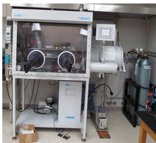
Fig. 4 Controlled atmosphere glove box that can maintain oxygen and moisture less than 2 ppm.
