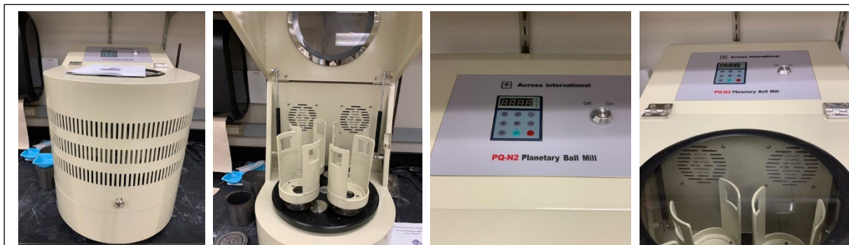
Fig. 3. Images of the planetary ball mill for preparation of the alloy matrix.
